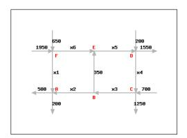
This can be modeled using a linear system of the form Ax = 0 with  $x = \begin{bmatrix} x_1 \\ x_2 \\ \vdots \\ x_6 \end{bmatrix}$ . At each data point, create an equation that maintains equilibrium. That is the input equals the output.
