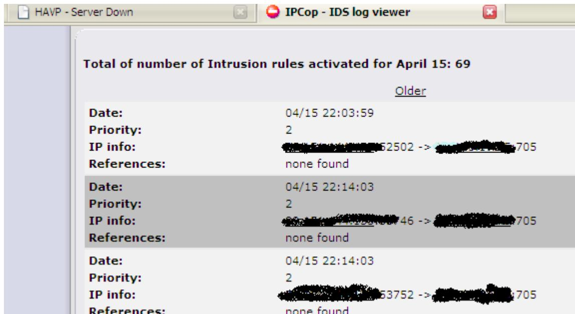
Figure 56. Snort IDS intrusion entry detail (Snort, 2007).
