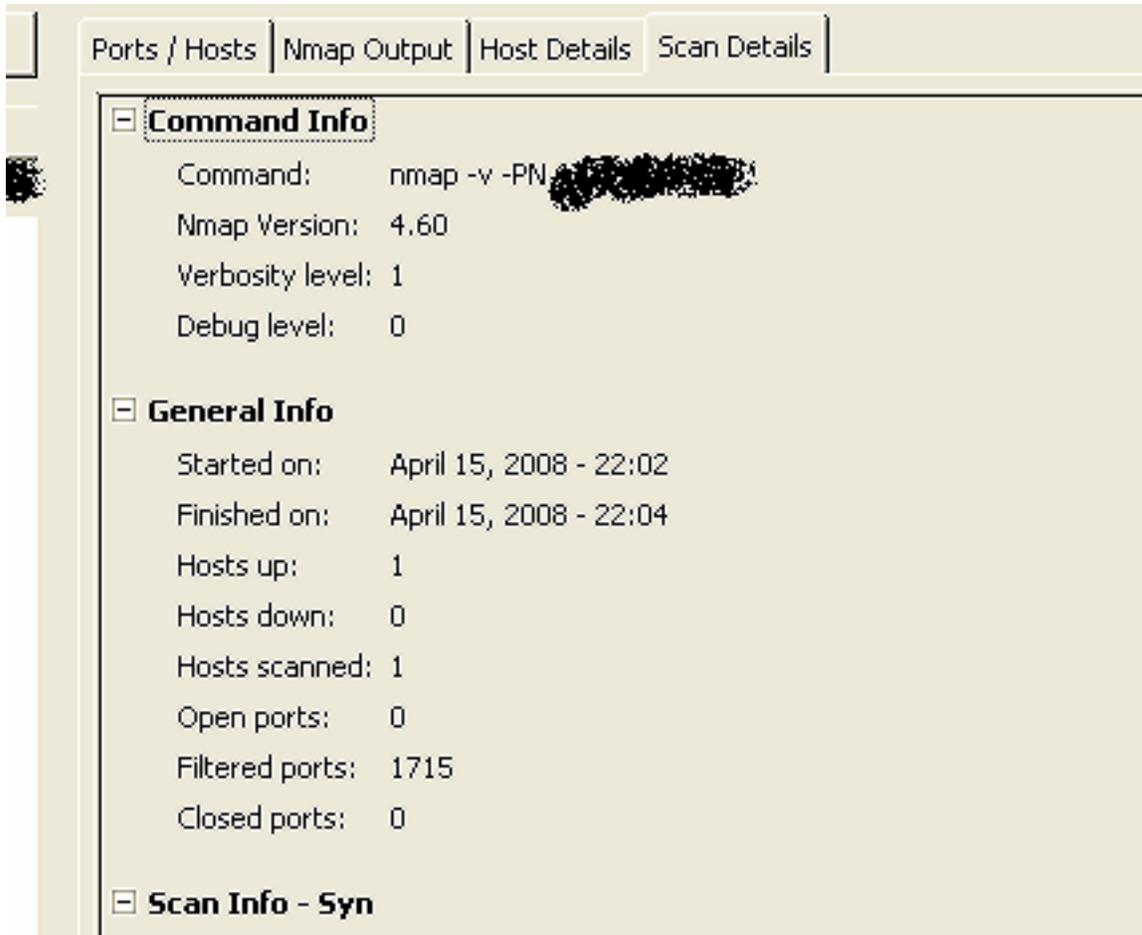
Figure 53. Zenmap regular scan details from our UTM configuration (Insecure.org, 2000).
