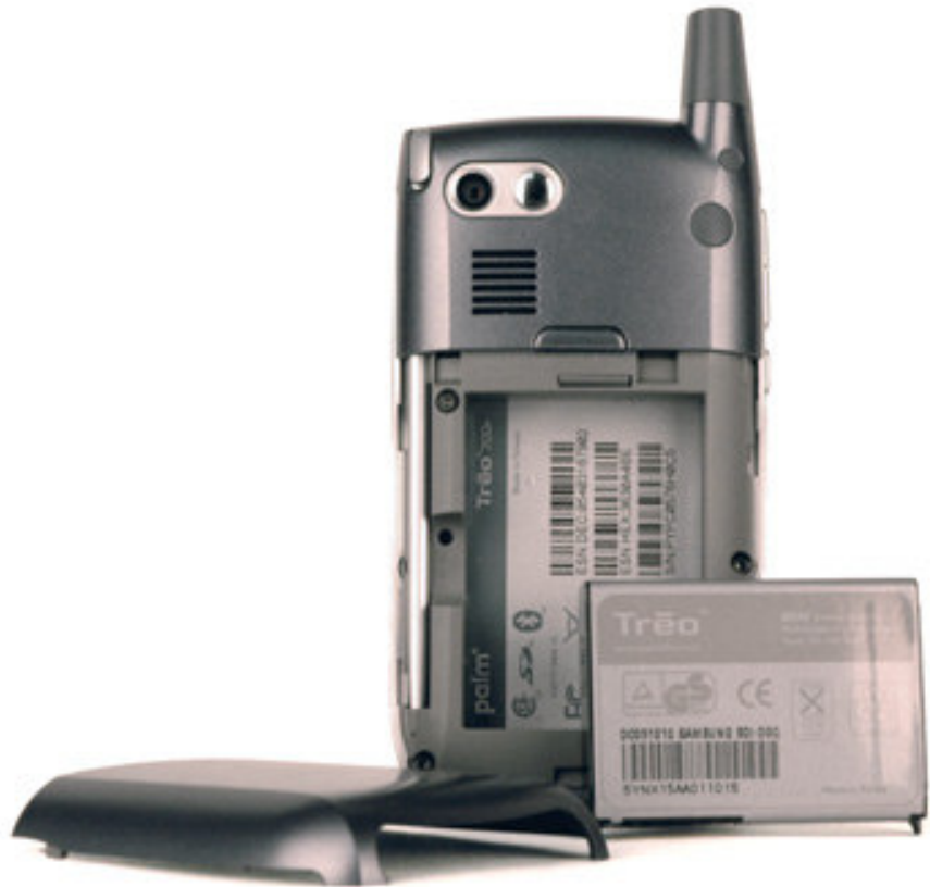
Figure 3. CDMA Treo showing no SIM Card Slot
